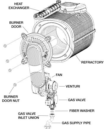
Figure 14.3: Exploded view of Heat Exchanger & Burner Assembly
