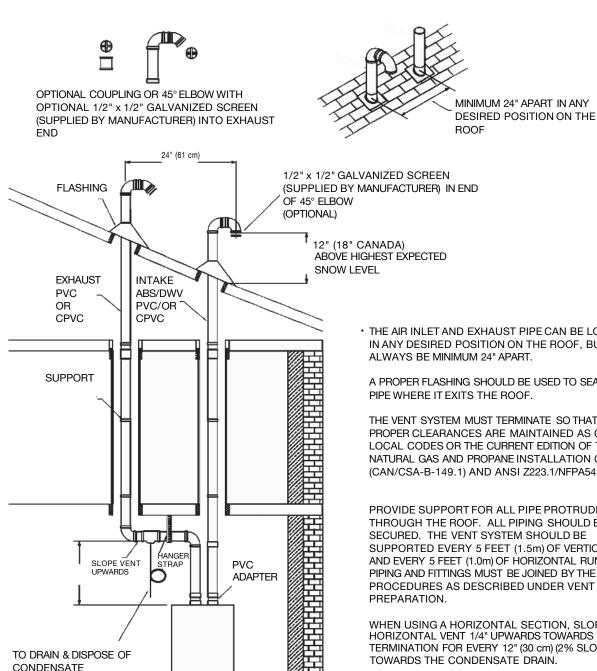
\* THE AIR INLET AND EXHAUST PIPE CAN BE LOCATED IN ANY DESIRED POSITION ON THE ROOF, BUT MUST
