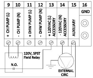
Figure 9.4: Field Connections External Voltage Source
