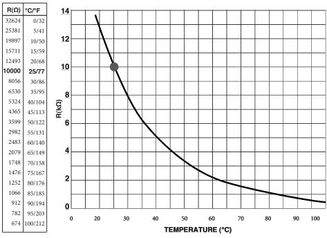
Table 12.3: Sensor Resistance Value Versus Temperature
