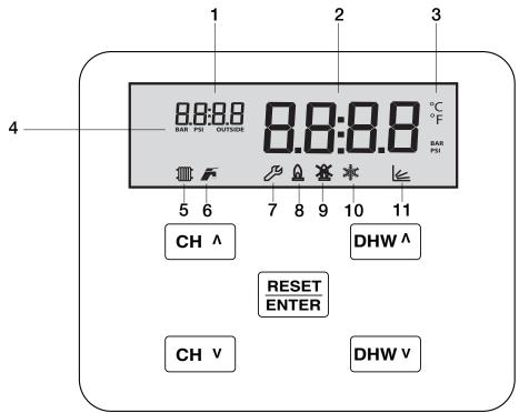
Figure 11.1: Combi LCD Display & Button Layout
