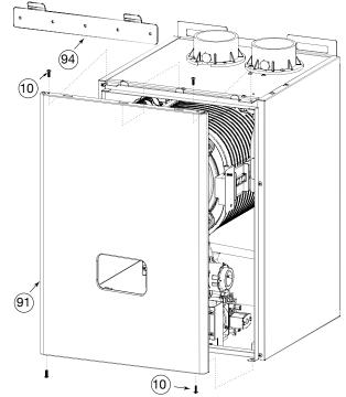
Figure 15.4: Front door Assembly
