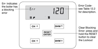
Figure 12.2: Blocking Error Display Screen
