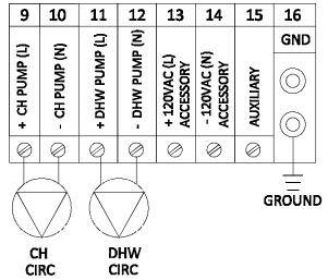
Figure 9.3: Field Connections Pumps Less Than 0.88 Amps Combined
