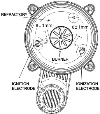
Figure 14.5: Burner Assembly Specifications
