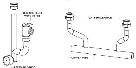
Figure 6.1: Pressure Relief Assembly
