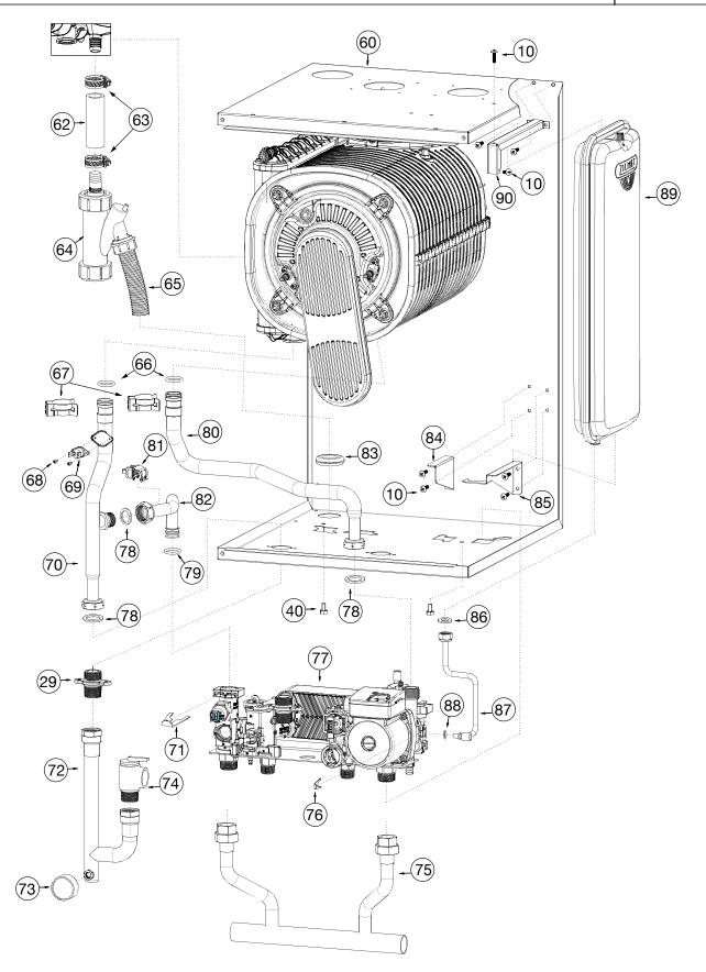
Figure 15.2: Cabinet Interior Wet Side Parts
