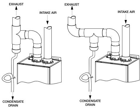
Fig 4.1: Vertical Drain Tee with Trap
