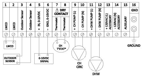
Figure 9.1: Simplified Wire Connections
