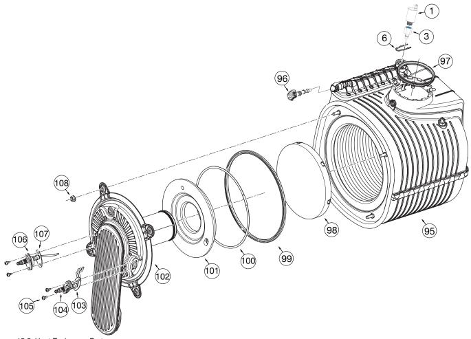
Figure 15.5: Heat Exchanger Parts
