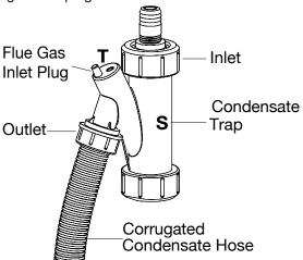
Figure 5.1: Condensate Drain
