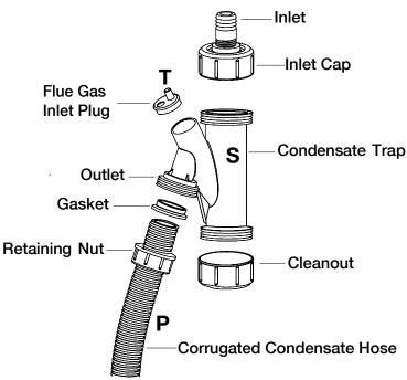
Figure 14.1: Condensate Drain
