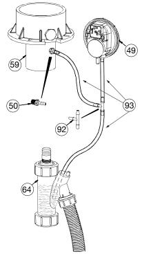
Figure 15.3: Blocked Flue Switch Loop
