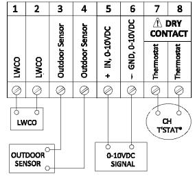
Figure 9.5: Field Connections Low Voltage
