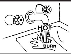
The temperature at which injury occurs varies with the person's age and time of exposure. Water temperature over 125°F/52°C can cause severe burns instantly or death from scalding.
