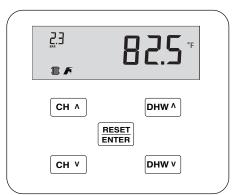
Figure 11.4: Main Screen in standby mode.
